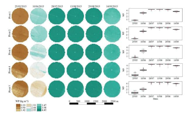
Figure 7. Water productivity of irrigated maize over the crop cycle in different central pivots.
