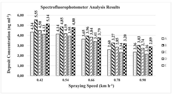
**Figure 8.** Average deposition of the mobile system at different spraying speeds for spraying locations A, B, C, D and E.
