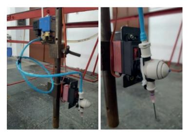
Figure 4. Servomotor coupled needle nozzle.
