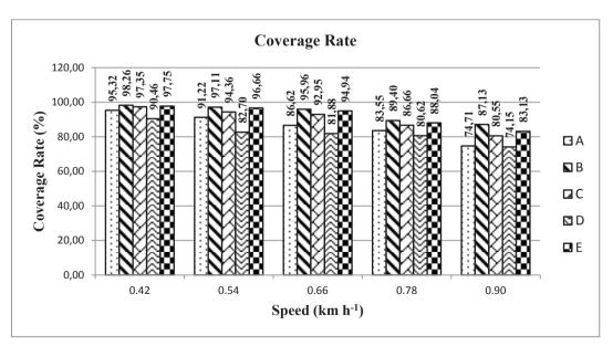
**Figure 10.** Coverage rate results of the steerable spraying needle nozzle at different spraying speeds for spraying locations A, B, C, D and E..
