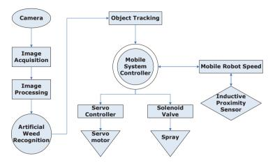
Figure 2. The system architecture of the mobile robot.
