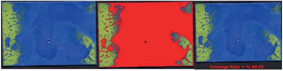
Original ImagePixel CountingCoverage RateFigure 9. The image-processing steps of a water-sensitive paper sample.
