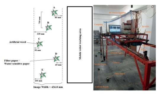
Figure 6. The layout of filter papers/water-sensitive papers attached to the artificial weeds and system design.
