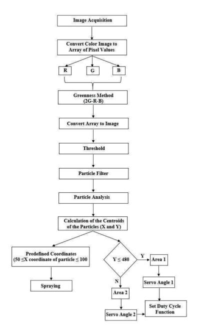
Figure 3. Image-processing and spraying procedure steps of the spraying system.
