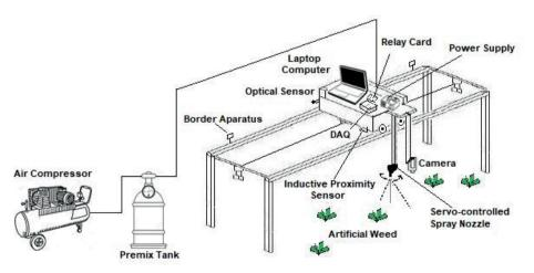
Figure 1. Schematic view of a servo-based target-oriented robotic weed control system.
