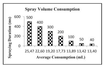
Figure 7. Spray volume consumption results of the system.
