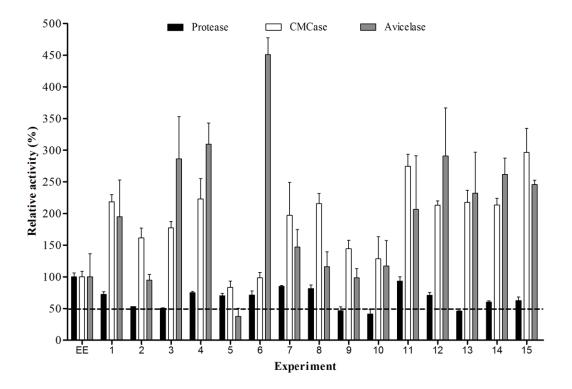
Note that all experiments had decreased proteolytic activity when compared to EE, though experiment 11 maintained activity levels above 90%. CMCase activity was sustained or increased by the drying process, and experiment 15 presented activity 3 times higher than EE. Avicelase activity was reduced in experiment 5 but was retained or improved in the others experiments, when compared to EE.
