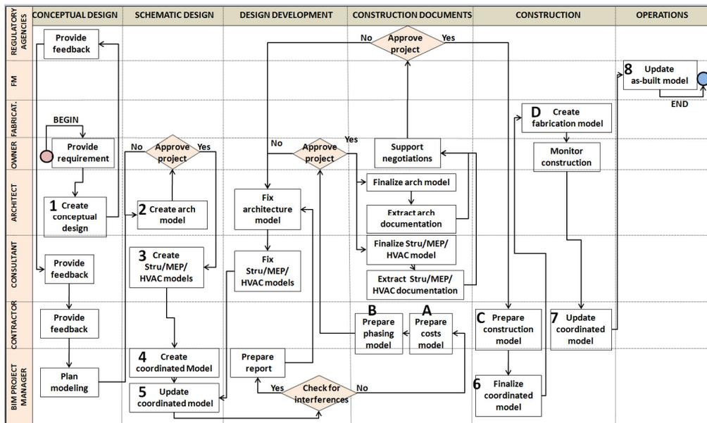
Figure 1 – Current BIM workflow used in Brazil by some AEC companies.
