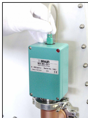
Insert plug connector.
