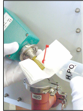
Moisten winding with phosphorous acid.
