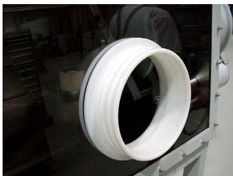
To replace the glove - place the glove over the port so that the rim of the glove locates in the port's innermost groove (the outer 2 grooves are for locating the O-rings that secure the glove).
