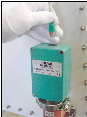
Disconnect plug connector.
